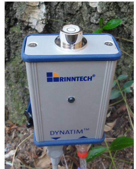
Inclination sensors at stem base and trunk head or structural timber
